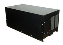
The MultiPhase converter is designed for use with CNC machines, machines with large inverters and all other three-phase machinery including welders. It reliably maintains the output voltage symmetry within narrow limits at all times and under all load conditions. The three-phase outputs provide pure 400V sine waves. Digital displays provide information on the output voltage and current.
